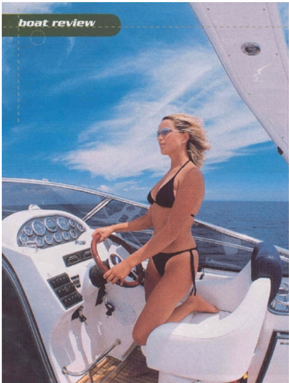
The helm area has a full range of analogue instrumentation, including: speedometer, rev counter, log, oil pressure, fuel level, hour counter, illuminated compass, and depth finder. Steering wheel and bucket seat are height adjustable.
