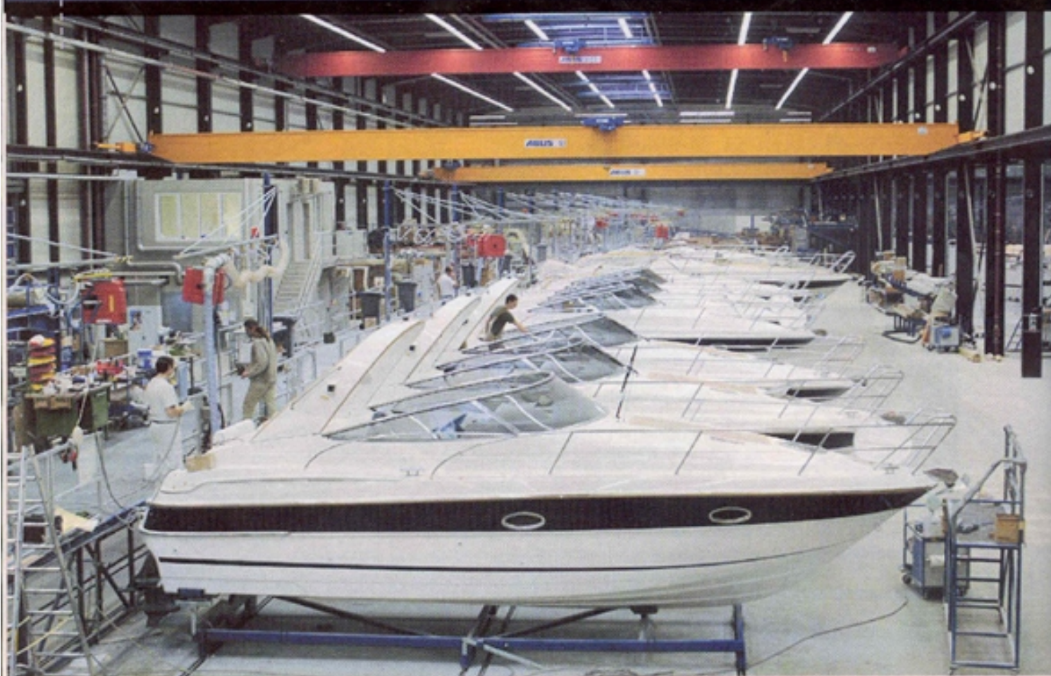
At station 30, the final stage, the boats are given their final touches and last pre-delivery inspection.
