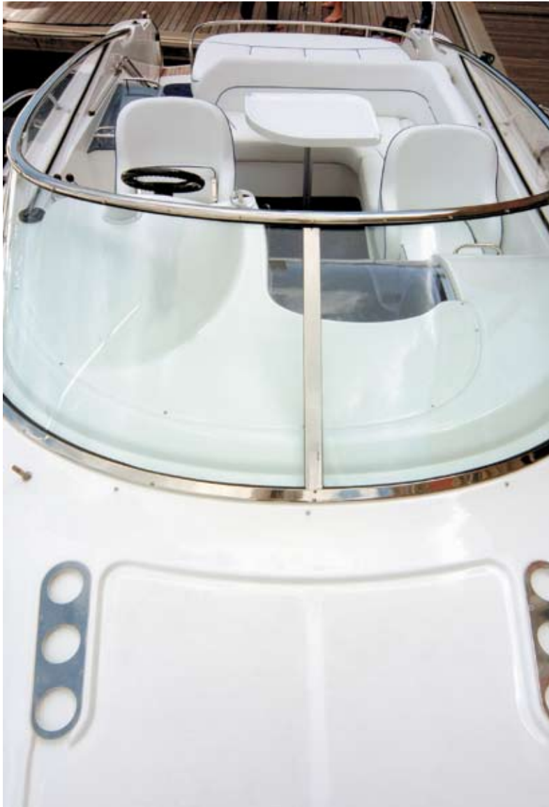
Wind protection comes in the form of a safety glass windscreen set into a stainless steel frame.
