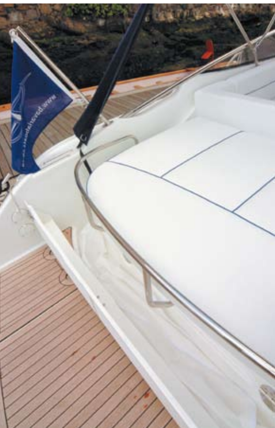
When not in use, the bimini frame folds into its own nifty aft storage compartment.
